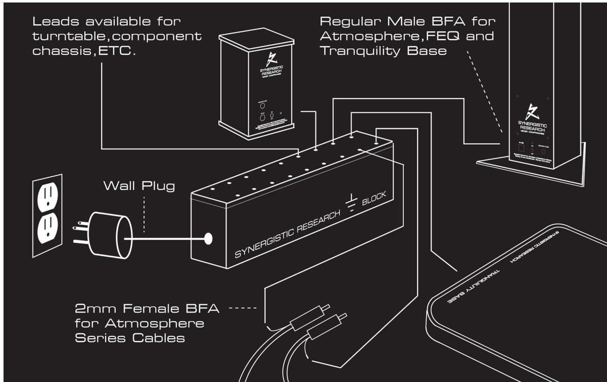
Grounding Block, High Def Grounding cable and standard grounding cable set up guide for use with components
